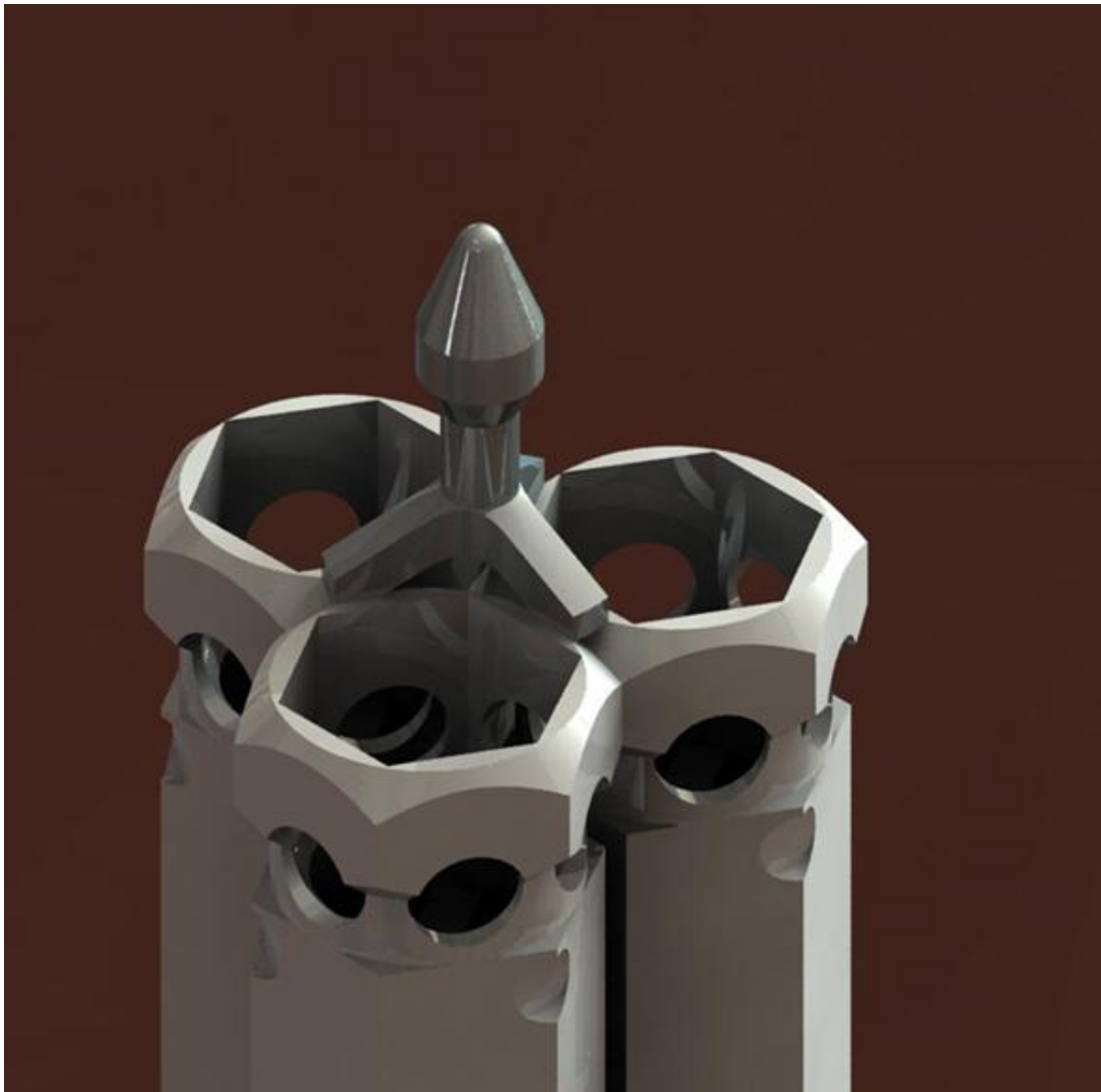
Figure 4-3: A VVR-M2 type triple fuel element.
